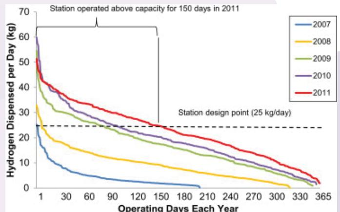
UCI Hydrogen Station Load duration Curve
